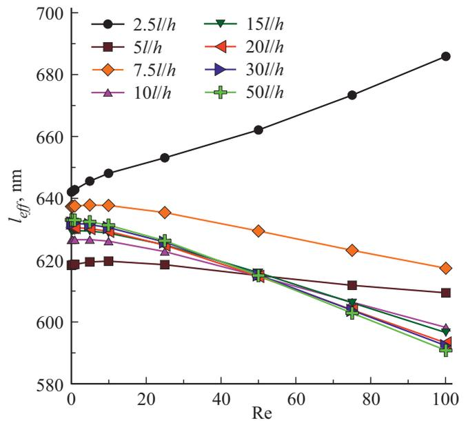
**Figure 2.** The dependence of the effective slip length on the microchannel wall on the Reynolds number for various relative lengths of such a microchannel.
