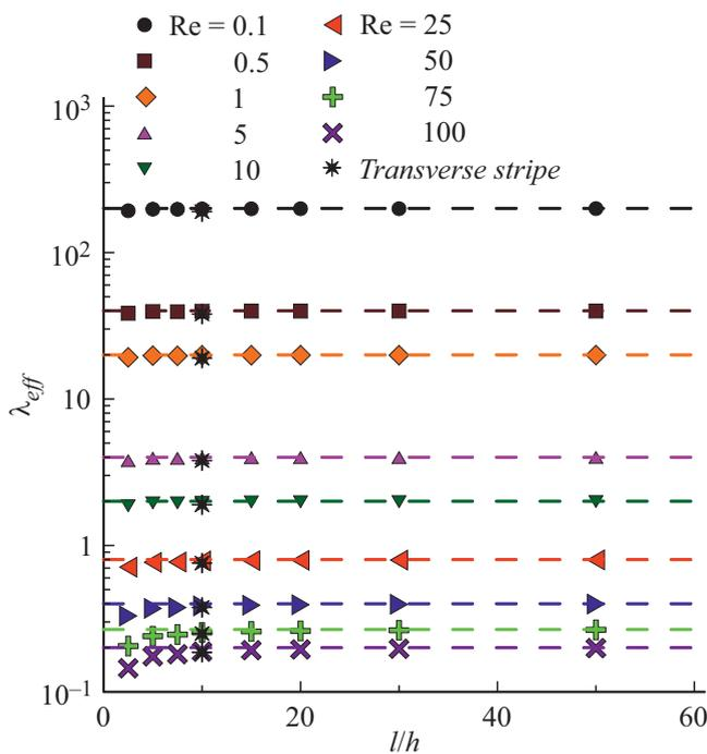
**Figure 3.** The dependence of the hydrodynamic friction factor on the relative length of the microchannel for various Reynolds numbers.
