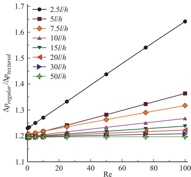
**Figure 1.** The dependence of the relative pressure drop in a microchannel on the Reynolds number for various relative lengths of such a microchannel.
