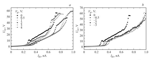
**Figure 7.** I–V characteristics of the SI GaAs sample passivated by sulfur under applied positive (*a*) and negative (*b*) gate-voltage T = 300 K.
