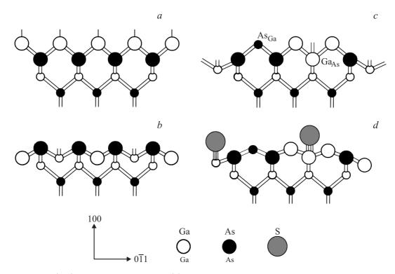
**Figure 8.** Model of the (100) face of the GaAs sample (*a*) reconstructed because of the negative-U properties for the Ga dangling bonds (*b*) and the Ga<sub>As</sub> double acceptor anti-site centers in the presence of the As<sub>Ga</sub> surface donor anti-site defects (*c*), which promote the sulfur adsorption processes (*d*).
