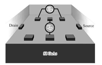
**Figure 2.** A device scheme designed to study the electrical properties of the surface of SI GaAs bulk. The I–V ( $U_{xx} = f(I_{ds})$ ) characteristics were measured under the gate voltage applied to the  $U_{xy}$  contacts.
