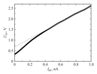
**Figure 3.** The I–V characteristic measured at the surface of the semi-insulating GaAs bulk structure. Solid line indicates the Coulomb blockade threshold,  $U_{th} = e/2C$ . T = 300 K.
