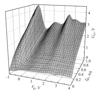
**Figure 4.** 3D plot of the Uxx voltage measured at the surface of the semi-insulating GaAs bulk structure at different values of the gate-voltage and the drain-source current. T = 300 K.
