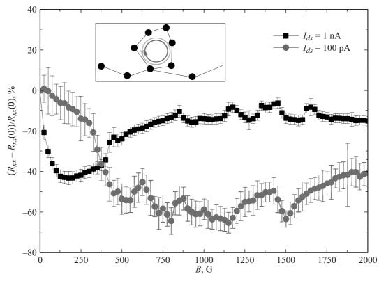
**Figure 10.** Relative magnetoresistance changes of the SI GaAs sample passivated by sulfur which were measured at two values of the drain-source current at T = 300 K. Insert: The loop containing series of scatters that result in the quantum interference between self-crossing paths in which an electron can propagate in the clock-wise and counter-clockwise direction.
