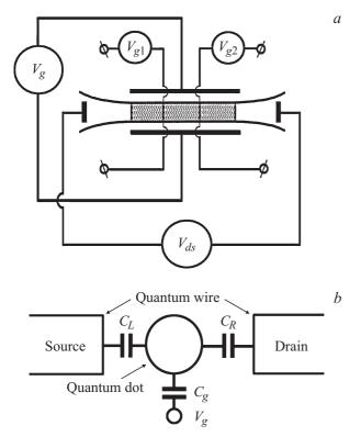
**Figure 1.** a — a schematic representation of the structure designed for studying the Coulomb blockade, Coulomb oscillations, and Coulomb staircase of the conductance of a quantum dot during the transport of single charge carriers. The split-gate voltage,  $V_g$ , is used to create the modulated QWr inside QW. The voltages  $V_{g1}$  and  $V_{g2}$  are applied to the finger gates to define a quantum dot. b — a scheme for a weakly coupled quantum dot inside a quantum wire.
