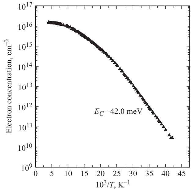
**Figure 1.** Charge carrier concentration versus reciprocal temperature for the  $n\text{-Si}_{1-x}\text{Ge}_x$  at  $x = 0.048$ . Points, experimental. Effective ionization energy of shallow donors is indicated.
