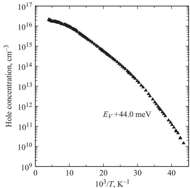
**Figure 2.** Charge carrier concentration versus reciprocal temperature for the  $p\text{-Si}_{1-x}\text{Ge}_x$  at  $x = 0.049$ . Points, experimental. Effective ionization energy of shallow acceptors is indicated.
