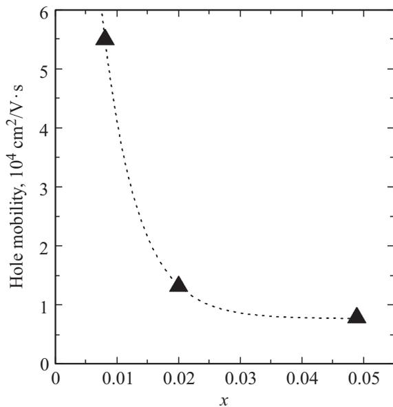
**Figure 6.** Partial mobility of holes due to alloy scattering at  $T \approx 28$  K versus mole fraction of Ge atoms  $x$  in the  $p$ - $\text{Si}_{1-x}\text{Ge}_x$  at  $x < 0.05$ . The dashed line is shown as the eye guide.
