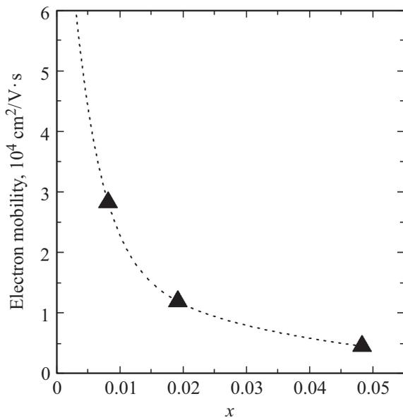
**Figure 5.** Partial mobility of electrons due to alloy scattering at  $T \approx 28$  K versus mole fraction of Ge atoms  $x$  in the  $n$ - $\text{Si}_{1-x}\text{Ge}_x$  at  $x < 0.05$ . The dashed line is shown as the eye guide.
