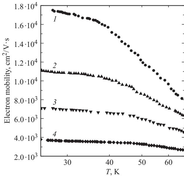
**Figure 3.** Charge carrier mobility versus temperature for the  $n\text{-Si}_{1-x}\text{Ge}_x$  at  $x < 0.05$ . Points, experimental:  $x = 0$  (1);  $x = 0.008$  (2);  $x = 0.019$  (3);  $x = 0.048$  (4).
