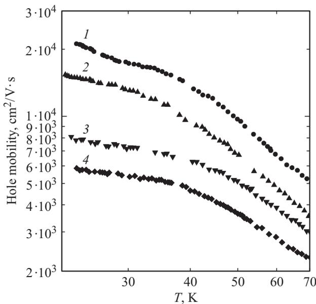
**Figure 4.** Charge carrier mobility versus temperature for the  $p\text{-Si}_{1-x}\text{Ge}_x$  at  $x < 0.05$ . Points, experimental:  $x = 0$  (1);  $x = 0.008$  (2);  $x = 0.02$  (3);  $x = 0.049$  (4).
