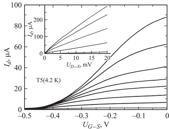
**Figure 3.** Example of characteristics of transistor T5 (from group *B*). Transient characteristics at  $T = 4.2\ \text{K}$  as a function of the magnetic field,  $B$ , equal to (from top to bottom, in Tesla):  $0$ ,  $0.030$ ,  $0.051$ ,  $0.068$ ,  $0.090$ ,  $0.140$ ,  $0.260$  and  $1$ . The inset shows output characteristics for gate-source voltage equal to (from top to bottom, in volts):  $0$ ,  $-0.1$ ,  $-0.2$ ,  $-0.3$  and  $-0.4$ .
