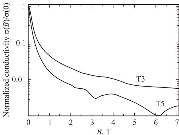
**Figure 7.** Magnetoconductance of the transistor T3 (upper curve) and T5 (lower curve).
