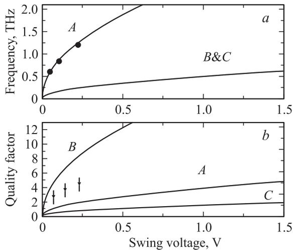
**Figure 10.** *a* — frequency of the resonant detection of the group A, B and C transistors, as a function of the swing voltage. *b* — quality factor corresponding to a frequency of the resonant detection, plotted in *a*), for the group A, B and C transistors.
