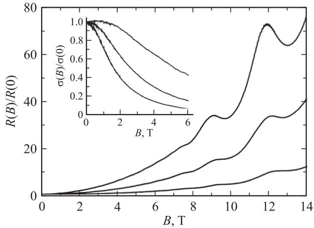
**Figure 4.** The resistance of a group A transistor, normalized at zero magnetic field, for  $U_{gs} = 0, 0.2$  and  $0.3$  V (from top to bottom). The inset shows normalized Lorentzian magnetoconductivity,  $\sigma(B)$ , curves characterized by decreasing  $\mu$  for increasing  $U_{gs}$ .
