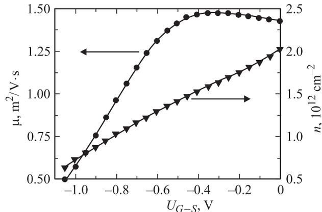
**Figure 9.** The electron mobility (squares) and concentration (down triangles) determined from measurements of the Hall effect on a gated Hall-bar of GaInAs/GaAlAs heterostructure from group C.
