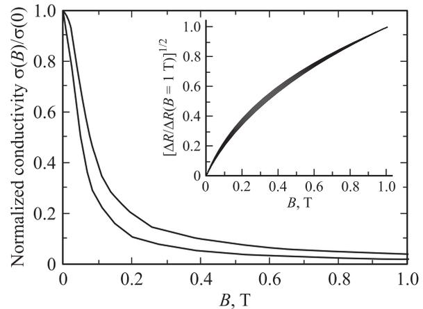
**Figure 5.** An influence of the magnetic field on conductivity for the transistor T3 (upper line) and T5 (lower line) — both transistors are from group B. The inset shows a square root of magnetoresistance  $\Delta R = R(B) - R(0)$  of the transistors T3 and T5, normalised to its value at 1 T. The curves correspond to gate-to-source voltage equal (in Volts) to 0,  $-0.1$ ,  $-0.2$ ,  $-0.3$ ,  $-0.4$  for T5 and 0,  $-0.1$ ,  $-0.2$ ,  $-0.3$  for T3.
