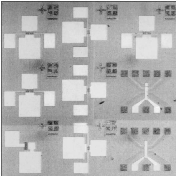
**Figure 2.** A photograph of a dice of the group *B* and *C* devices with lithographically defined six transistors, two Hall-bars and Schottky diode.
