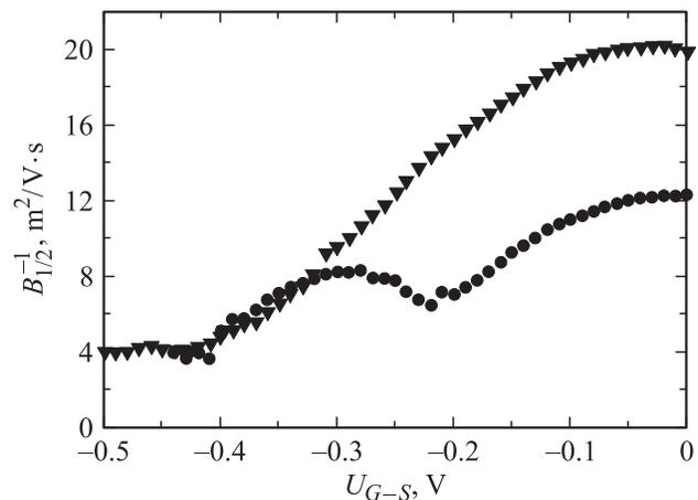
**Figure 6.** An inverse of the halfwidth of magnetoconductivity curves,  $B_{1/2}^{-1}$ , for the transistors T5 ( $L = 1.5 \mu\text{m}$ , down triangles) and T3 ( $L = 2.5 \mu\text{m}$ , solid circles), as a function of gate-to-source voltage,  $U_{gs}$ .
