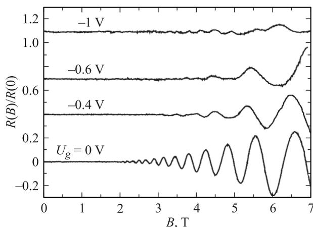
**Figure 8.** Shubnikov–de Haas oscillations of magnetoresistance of a Hall-bar processed out of GaInAs/GaAlAs heterostructure (group C of devices), as a function of the magnetic field, for gate potential equal to 0, 0.4, 0.6 and 1 V (from bottom to top). The curves are normalized at  $B = 0$  T and shifted vertically for a better visualization.
