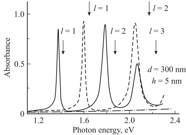
**Figure 3.** Absorption spectra of light incident normally onto a silver surface with spherical inclusions of a material with dielectric constant  $\epsilon = 4.5$  (solid curve) and  $\epsilon = 3.3$  (dashed curve). The absorption of light on the surface of bulk silver is shown by dash-dotted curve. Vertical arrows mark the energies of the fundamental ( $l = 1$ ), second ( $l = 2$ ), and third ( $l = 3$ ) plasmon modes of a single void in bulk silver.
