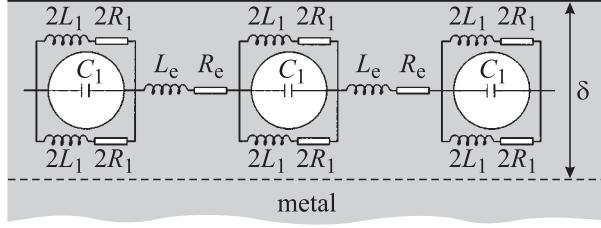
**Figure 1.** Nanoporous surface of metal and its equivalent circuit.
