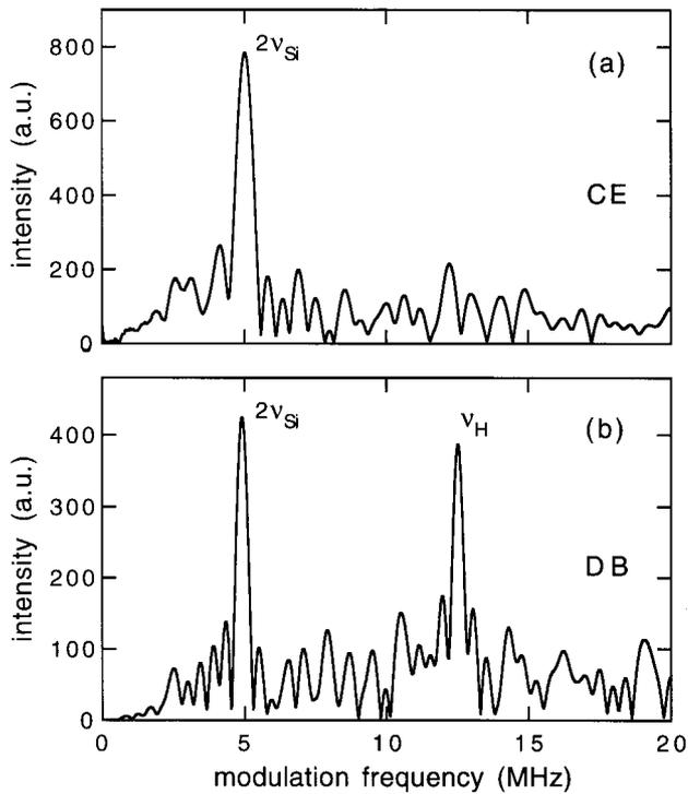
**Figure 1.** Fourier transform ESEEM spectra for CE (a) and DB (b) in  $\mu c$ -Si:H.
