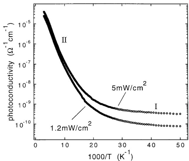
**Figure 3.** Temperature dependences of the photoconductivity at two light intensities.
