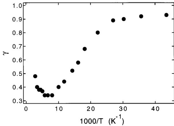
**Figure 4.** Temperature dependence of the exponent  $\gamma$  in the relation  $\sigma_p \propto F^\gamma$ .
