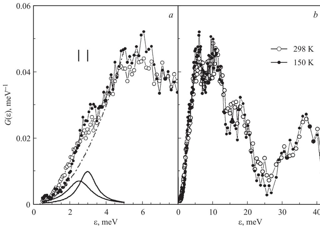
**Figure 2.** Low-energy part (a) and complete (b)  $G(\varepsilon)$  in AgCuS at  $T = 150$  and  $298$  K (KDSOG-M measurements). The low-energy part of the  $G(\varepsilon)$  with fitting by a superposition of Debye law (dot dashed line) and Lorentzian function (solid line) are shown in part a. Vertical marks correspond to the center of Lorentzian function at  $T = 150$  and  $298$  K.
