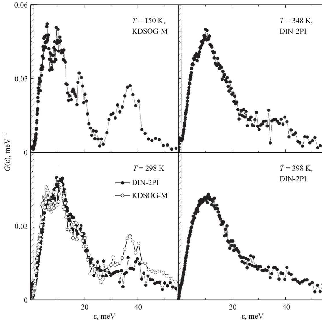
**Figure 1.** Spectra of  $G(\varepsilon)$  at  $T = 150, 298, 348$  and  $398$  K (KDSOG and DIN-2PI measurements).
