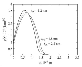
**Figure 4.** Electron wave functions based on proposed model for devices with  $N_A = 10^{17} \text{ cm}^{-3}$ ,  $V_{\text{GB}} = 0.93 \text{ V}$ .
