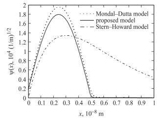
**Figure 3.** The electron wave function for a NMOS with  $N_A = 4 \cdot 10^{14} \text{ cm}^{-3}$ ,  $t_{\text{ox}} = 2.3 \text{ nm}$  and  $V_{\text{GB}} = 0.62 \text{ V}$  obtained from the proposed model (solid), the Stern–Howard [15] model (dash-dotted line) and the Mondal–Dutta model [8] (dotted).
