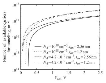
**Figure 5.** The number of electrons for various substrate doping concentrations and oxide widths.
