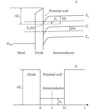
**Figure 2.** *a* — band diagram of the NMOS structure and *b* — the obtained symmetric rectangular potential well after simplifications.
