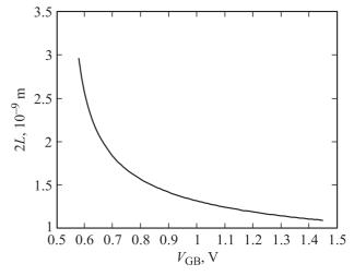
**Figure 7.** Inversion layer thickness 2*L* as a function of the applied gate-to-body voltage  $V_{\rm GB}$  for a device having  $N_A = 8.5 \cdot 10^{17} \, {\rm cm}^{-3}$  and  $t_{\rm ox} = 2.3 \, {\rm nm}$ .
