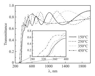
**Fig. 6.** Transmittance of ZnS films deposited at various substrate temperature. Inset shows the effect of substrate temperature on the absorption edge.
