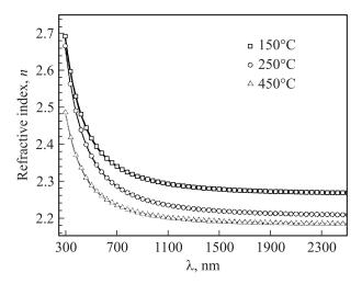
**Fig. 5.** Refractive indices of ZnS films deposited at various substrate temperature.
