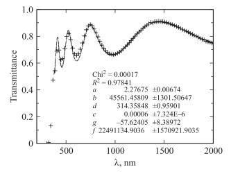
**Fig. 3.** Transmittance data of a ZnS film deposited at the substrate temperature  $350^{\circ}$ C along with the fitted curve (solid line).
