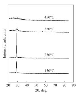
**Fig. 1.** XRD pattern of ZnS films deposited at various substrate temperatures.
