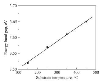
**Fig. 4.** Variation of energy bandgap of ZnS films deposited at various substrate temperatures. Solid line is linear fit to the data points.
