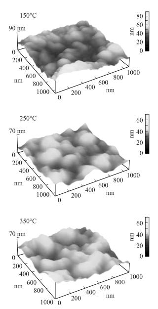
**Fig. 2.** AFM images of ZnS films deposited at the substrate temperatures of 150, 250 and  $350^{\circ}$ C.
