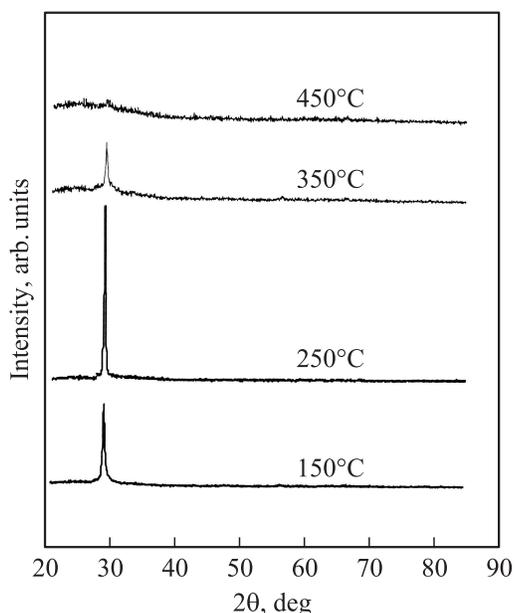
**Fig. 1.** XRD pattern of ZnS films deposited at various substrate temperatures.
