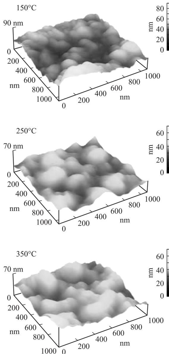
**Fig. 2.** AFM images of ZnS films deposited at the substrate temperatures of 150, 250 and 350°C.
