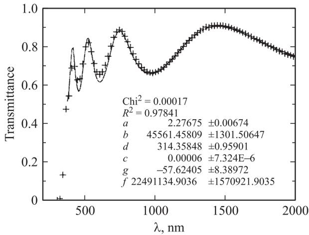
**Fig. 3.** Transmittance data of a ZnS film deposited at the substrate temperature 350°C along with the fitted curve (solid line).
