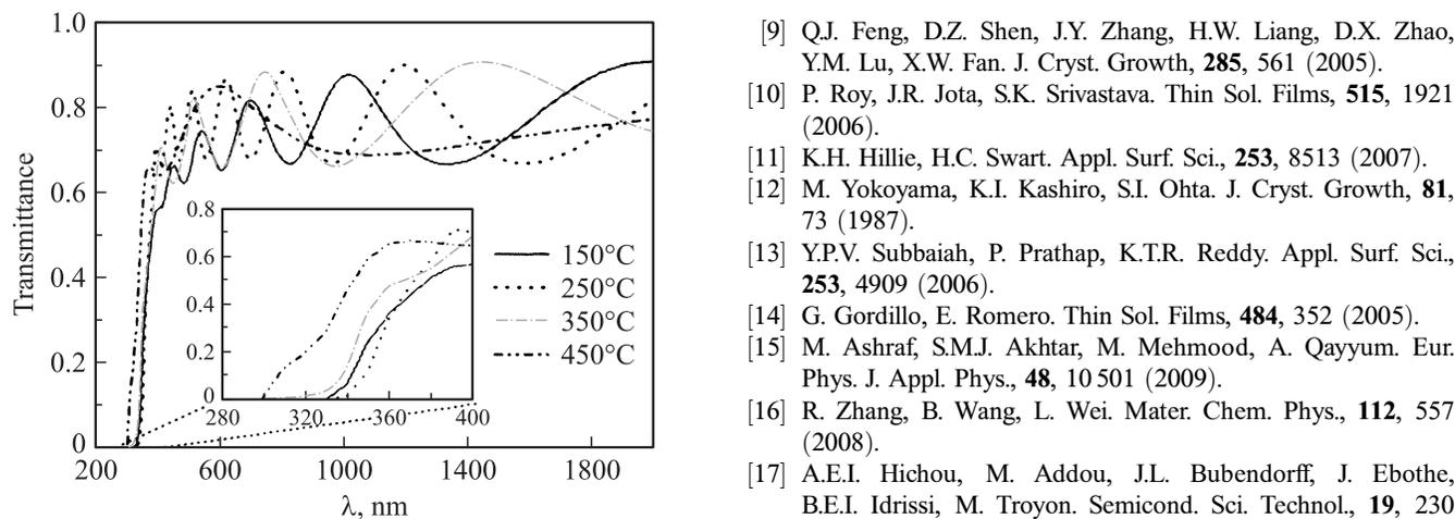
**Fig. 6.** Transmittance of ZnS films deposited at various substrate temperature. Inset shows the effect of substrate temperature on the absorption edge.
