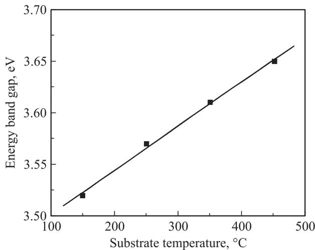
**Fig. 4.** Variation of energy bandgap of ZnS films deposited at various substrate temperatures. Solid line is linear fit to the data points.
