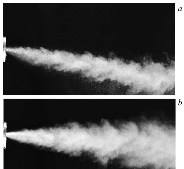
Figure 2. Path of a water jet at small degrees of superheating corresponding to the following temperatures in the working chamber: T_s = 140 ( a ) and 160^\circ\text{C} ( b ).
