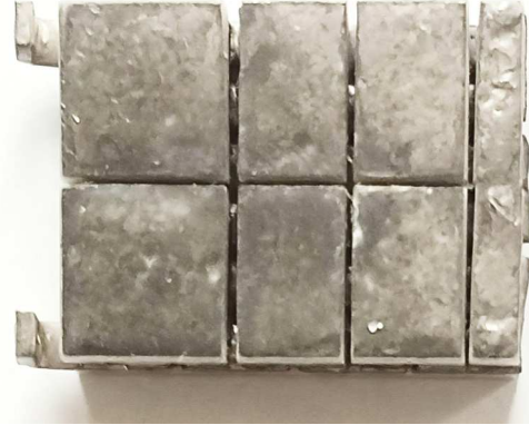
Figure 3. Outside view of the cooler with tinned cooling surface.
