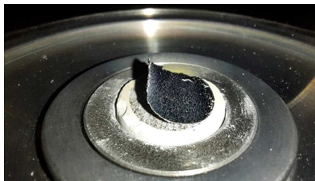
Figure 9. Target pressed without sintering after laser exposure. Full separation of the molten surface layer from the main target body is obvious.
