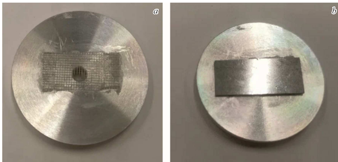
Figure 5. Sample holder photograph: a — with attached masking mesh; b — with attached sample.
