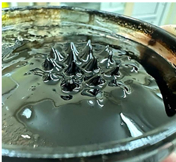
Figure 1. Image of the FLG-based magnetic composite material exposed to a magnetic field.
