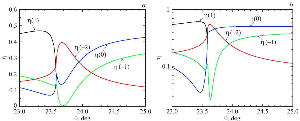
**Figure 3.** a — Absolute diffraction efficiency ( $\eta$ ) of the  $0.6 \text{ mm}^{-1}$   $\text{Al}_{0.3}\text{Ga}_{0.7}\text{As}$  grating with symmetric triangular grooves with an angle of  $18.3^\circ$  at a wavelength of  $1000 \mu\text{m}$  in TM polarization at a temperature of 30 K as a function of incidence angle  $\theta$ ; b —  $\eta(n)$  of the same grating, but with a perfect conductivity.
