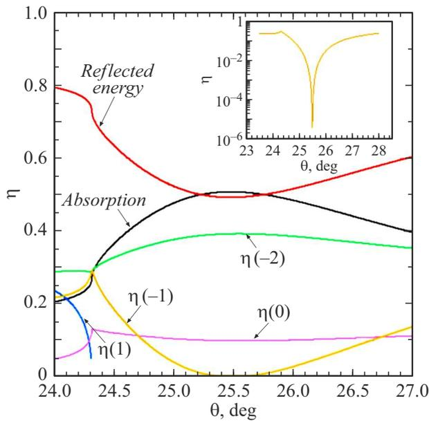
**Figure 2.** Absolute diffraction efficiency ( $\eta$ ) of the  $0.588 \text{ mm}^{-1}$  GaAs grating with symmetric triangular grooves with angle  $24.7^\circ$  at a wavelength of  $1000 \mu\text{m}$  in TM polarization at a temperature of 30 K as a function of incidence angle  $\theta$ . The inset presents  $\eta(-1)$  in logarithmic scale.
