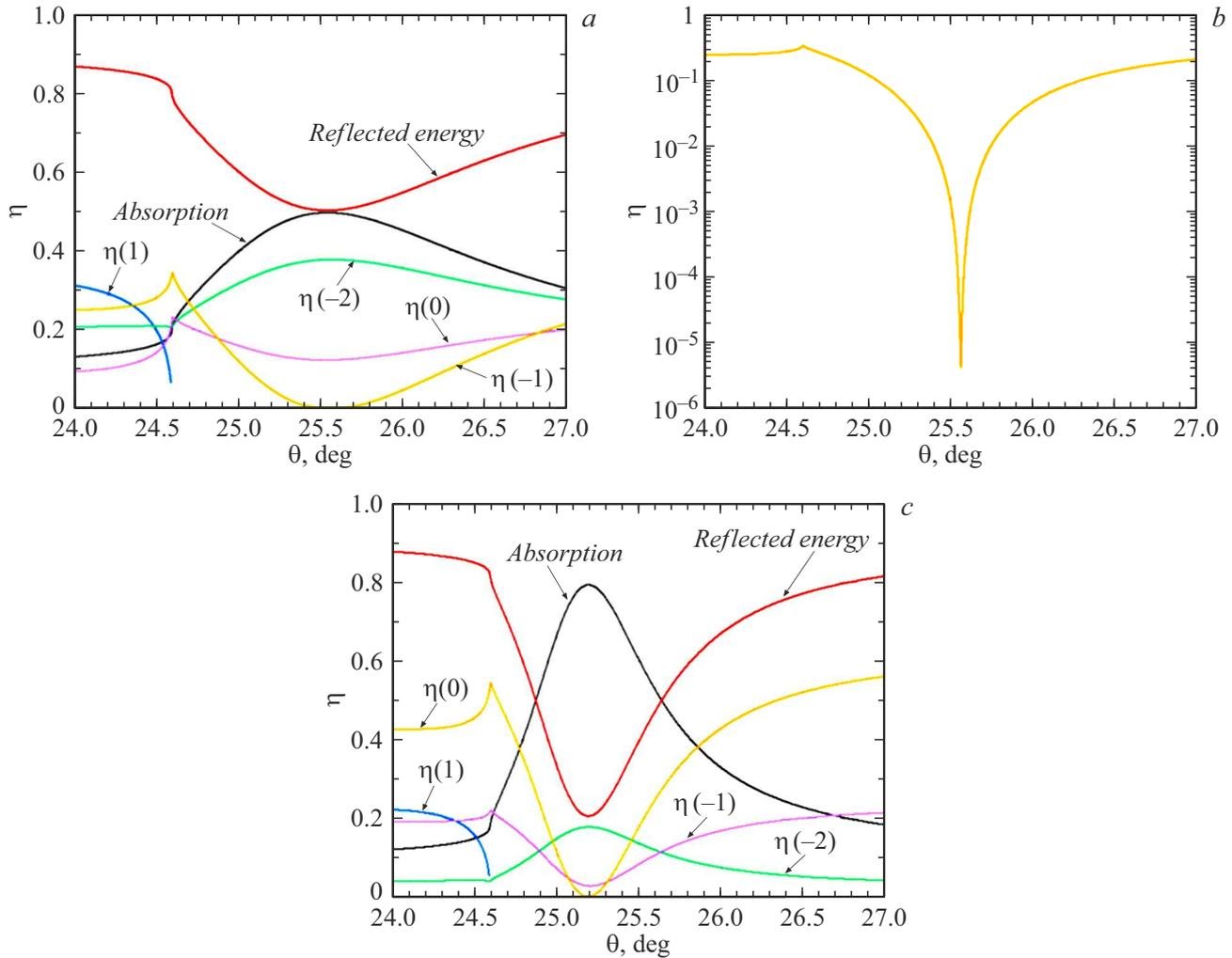
**Figure 1.** Absolute diffraction efficiency of orders ( $\eta$ ) of the 1.946 mm<sup>-1</sup> InSb grating with symmetric triangular grooves at a wavelength of 300  $\mu$ m in TM polarization as a function of incidence angle  $\theta$ . *a* —  $\eta(n)$  for triangle angle  $\alpha = 21.6^\circ$ ; *b* —  $\eta(-1)$  in logarithmic scale for triangle angle  $\alpha = 21.6^\circ$ ; and *c* —  $\eta(n)$  for triangle angle  $\alpha = 13.1^\circ$ .
