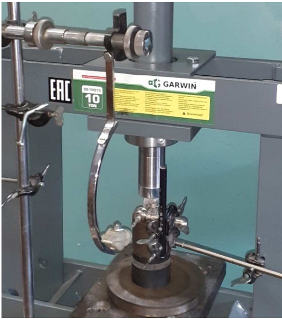
Figure 1. Photo of a setup for generating AE in case of impact damage to a uniaxially compressed sample CS.
