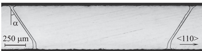
Figure 2. Photograph of a cross-section of a closed cell formed by an annular zone. The cross section is in the direction of \langle 110 \rangle along the diameter of the zone. The finish surface of the wafer is at the bottom. TM process temperature is 1300 K.
