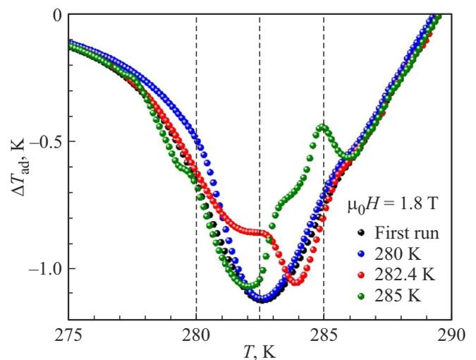
**Figure 9.** MCE vs. temperature in  $\text{Ni}_{43.18}\text{Mn}_{45.15}\text{In}_{11.67}$  in 1.8 T field after the measurements at fixed temperature, and the initial curve.
