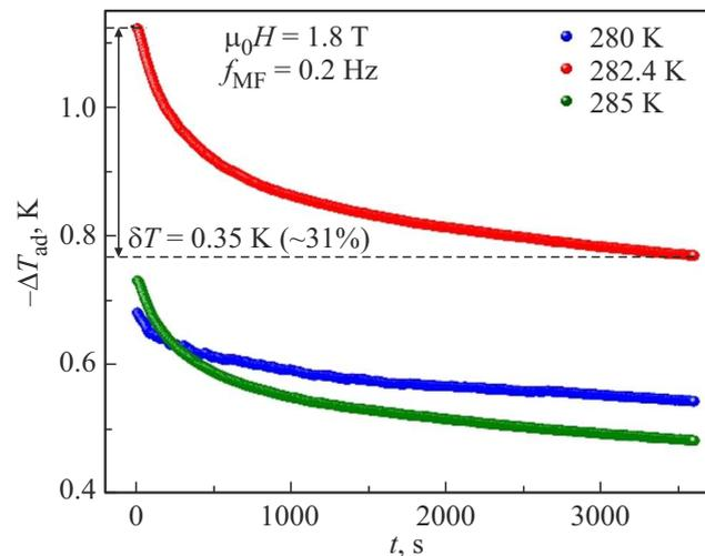
**Figure 7.** MCE vs. temperature in  $\text{Ni}_{43.18}\text{Mn}_{45.15}\text{In}_{11.67}$  in 1.8 T cyclic magnetic field in the magnetostructural phase transition region.
