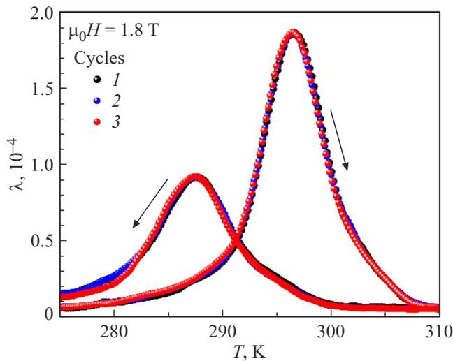
**Figure 6.** Magnetostriction vs. temperature in  $\text{Ni}_{43.18}\text{Mn}_{45.15}\text{In}_{11.6}$  in 1.8 T magnetic field.
