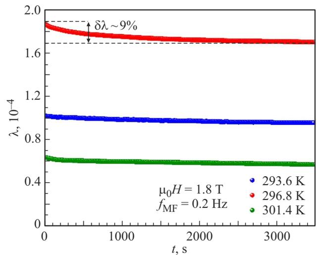
**Figure 8.** Magnetostriction vs. temperature in  $\text{Ni}_{43.18}\text{Mn}_{45.15}\text{In}_{11.67}$  in 1.8 T cyclic magnetic field in the magnetostructural phase transition region.
