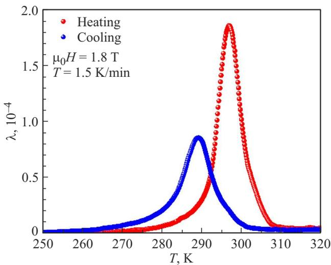
**Figure 4.** Magnetostriction vs. temperature in  $\text{Ni}_{43.18}\text{Mn}_{45.15}\text{In}_{11.67}$  in the cyclic magnetic fields with an amplitude of 1.8 T during heating and cooling runs.
