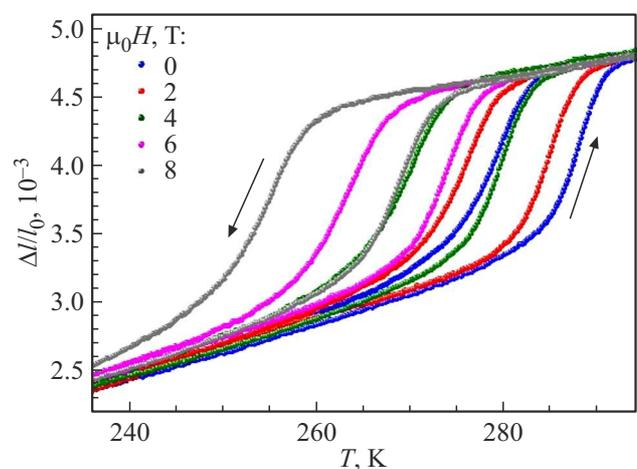
**Figure 2.** Linear thermal expansion vs. temperature of  $\text{Ni}_{43.18}\text{Mn}_{45.15}\text{In}_{11.67}$  in various magnetic fields during heating and cooling runs.
