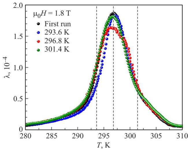
**Figure 10.** Magnetostriction vs. temperature in  $\text{Ni}_{43.18}\text{Mn}_{45.15}\text{In}_{11.67}$  in 1.8 T field after the measurements at fixed temperature, and the initial curve.
