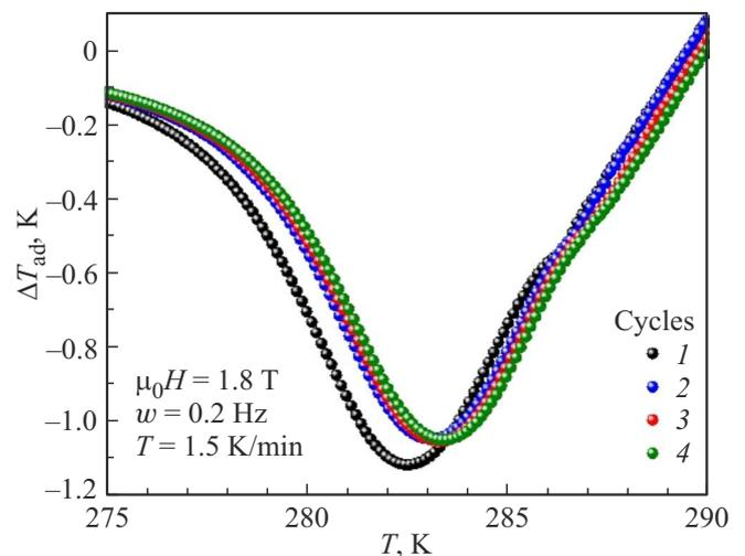
**Figure 5.** MCE vs. temperature in  $\text{Ni}_{43.18}\text{Mn}_{45.15}\text{In}_{11.6}$  in 1.8 T magnetic field.
