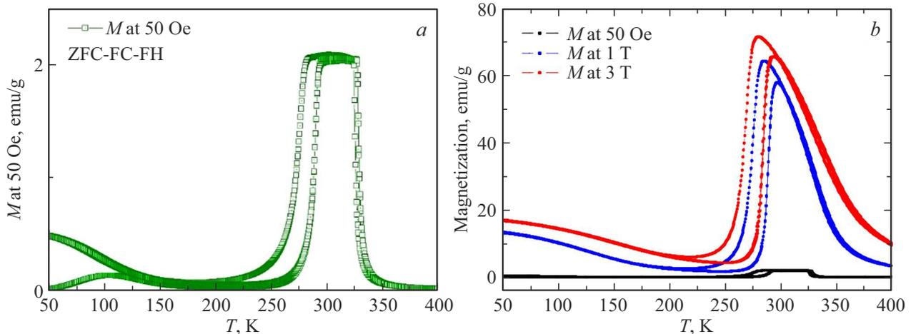
**Figure 1.** Alloy magnetization  $\text{Ni}_{43.18}\text{Mn}_{45.15}\text{In}_{11.67}$  in magnetic fields up to 3 T.
