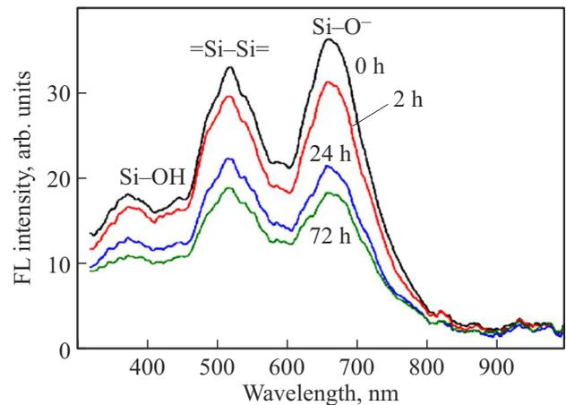
**Figure 1.** PL spectra of samples before and after the FA. The annealing duration is shown near the spectra.
