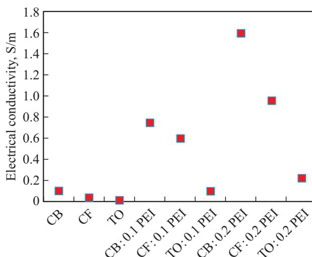
**Figure 2.** Electrical conductivity of doped and non-doped samples.
