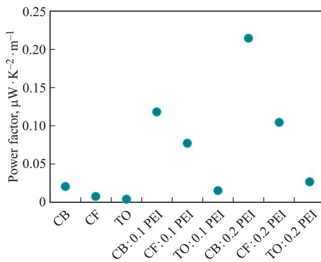
**Figure 4.** Power factor values of doped and non-doped samples.
