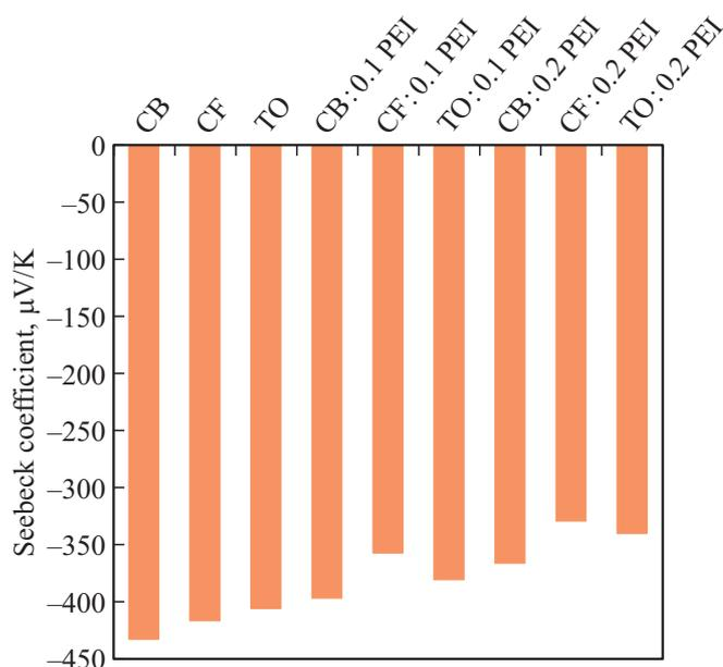
**Figure 3.** Seebeck coefficient values of doped and non-doped samples.
