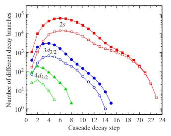
**Figure 1.** The number of different decay tree branches that appear at successive decay steps for the cascades with initial vacancies in the 2s-,  $3d_{3/2}$ - and  $4d_{3/2}$ -subshells of the gold atom. Empty symbols — calculation without taking SO processes into account, solid symbols — calculation taking SO processes into account.
