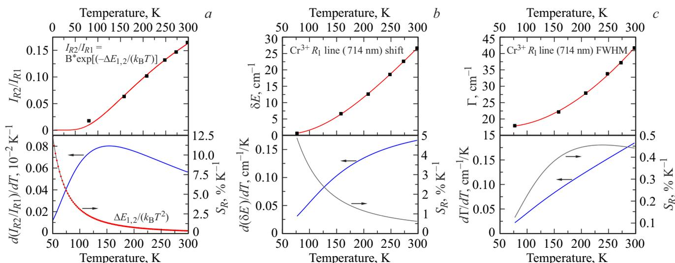
**Figure 10.** Upper row: temperature dependences of the ZPL intensity ratio at 700 and 714 nm (a), ZPL spectral shift at 714 nm (b), ZPL full width at half maximum at 714 nm (c). The lines show the results of the experimental data approximation (points) by the Boltzmann function (a) and the McComber & Sturge [25] (b and c) formulas. Lower row: temperature dependences of sensitivity (left) and relative sensitivity (right,  $S_R$ ) of each of the temperature measurement methods.
