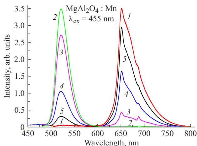
**Figure 2.** Luminescence spectra of manganese ions in  $\text{MgAl}_2\text{O}_4$  samples synthesized under different conditions, in particular, the (1) — sample using a multistage annealing procedure at 500, 600, 700, 1000, 1200, and 1300°C in air, sample (2) — in a reducing CO atmosphere, samples (3–5) — synthesized in air at temperatures of 1000, 1200, and 1300°C, respectively without pre-annealing at lower temperatures.
