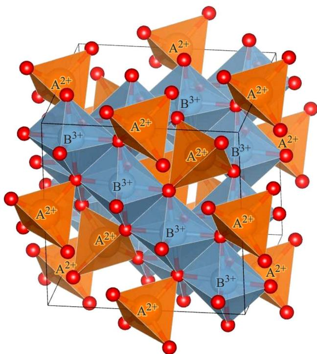
**Figure 1.** Crystal structure of spinel. In this example, the divalent cations  $A^{2+}$  occupy tetrahedral positions, and the trivalent cations  $B^{3+}$  occupy octahedral sites in  $AB_2O_4$ , as is observed in the structures of normal spinels  $MgAl_2O_4$  and  $ZnAl_2O_4$ .
