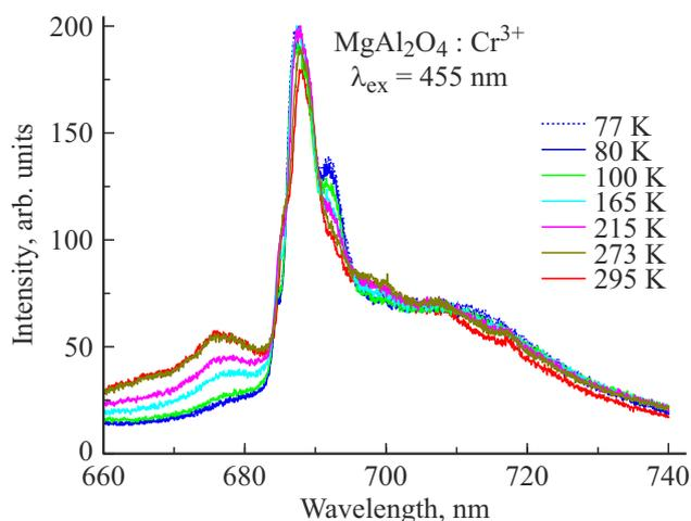
**Figure 3.** Luminescence spectra of  $\text{MgAl}_2\text{O}_4:\text{Cr}^{3+}$  measured at different temperatures.
