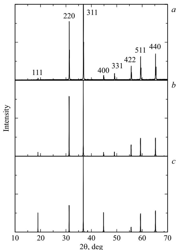
**Figure 4.** (a) Experimental X-ray diffraction pattern of the synthesized spinel sample  $\text{ZnAl}_2\text{O}_4$ ; (b) X-ray diffraction pattern of  $\text{ZnAl}_2\text{O}_4$  spinel from the database [17]; (c) simulated X-ray diffraction pattern of inverse spinel  $\text{ZnAl}_2\text{O}_4$ .
