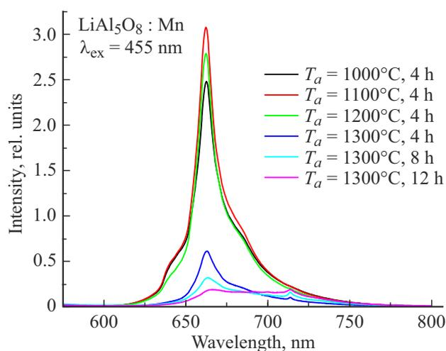
**Figure 8.** Luminescence spectra of  $\text{Mn}^{4+}$  ions in  $\text{LiAl}_5\text{O}_8$  ceramic samples synthesized at annealing temperatures of 1000, 1100, 1200, and 1300°C and annealing times of 4, 8, and 12 h.
