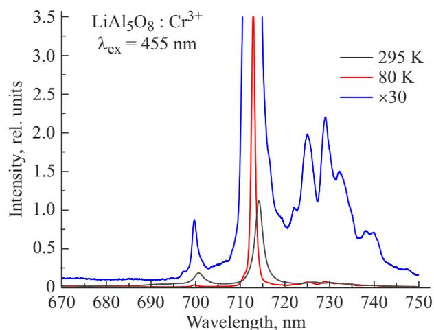
**Figure 9.** Luminescence spectrum of ceramics  $\text{LiAl}_5\text{O}_8:\text{Cr}^{3+}$  (0.1 at.%) measured at 80 and 295 K. The spectrum at 80 K is also shown on an enlarged scale to demonstrate the structure of the vibronic (Stokes) lines related to the ZPL at 714 nm.
