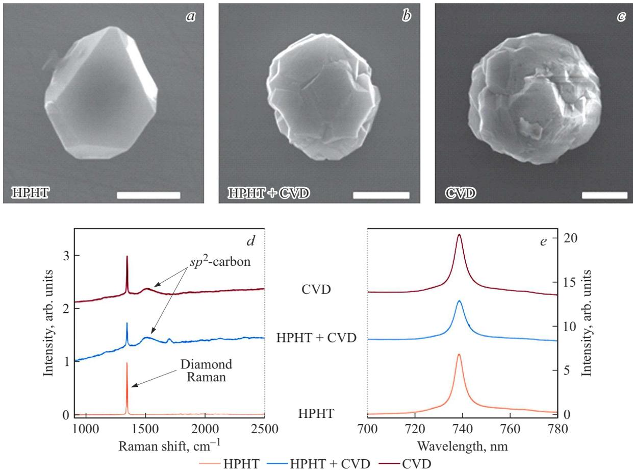
**Figure 1.** Representative SEM images of diamond (a) HPHT-, (b) (HPHT+CVD)- and (c) CVD microparticles. The scale line in the bottom right corner corresponds to  $1\mu\text{m}$ . (d, e) Corresponding Raman and luminescence spectra of SiV centers at 473-nm excitation, obtained at room temperature. ( $23^\circ\text{C}$ ).
