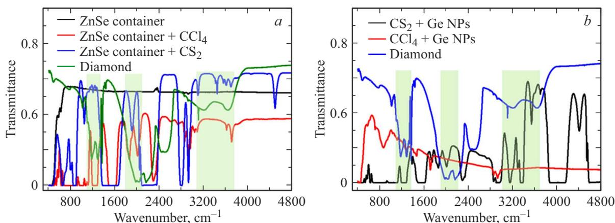
**Figure 5.** IR spectra of a cell made of ZnSe and with the addition of liquid carbon disulfide and carbon tetrachloride (a), germanium nanoparticles dissolved in carbon disulfide and carbon tetrachloride (b), in comparison with the spectrum of diamond.
