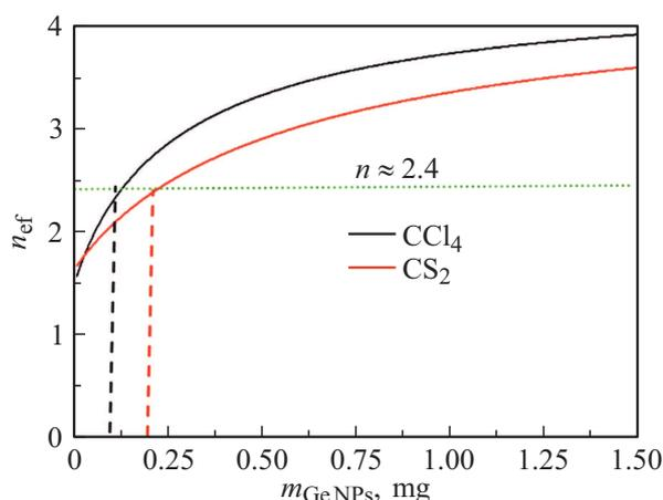
**Figure 3.** Dependence of the effective refractive index of the immersion medium on the mass of germanium nanoparticles.
