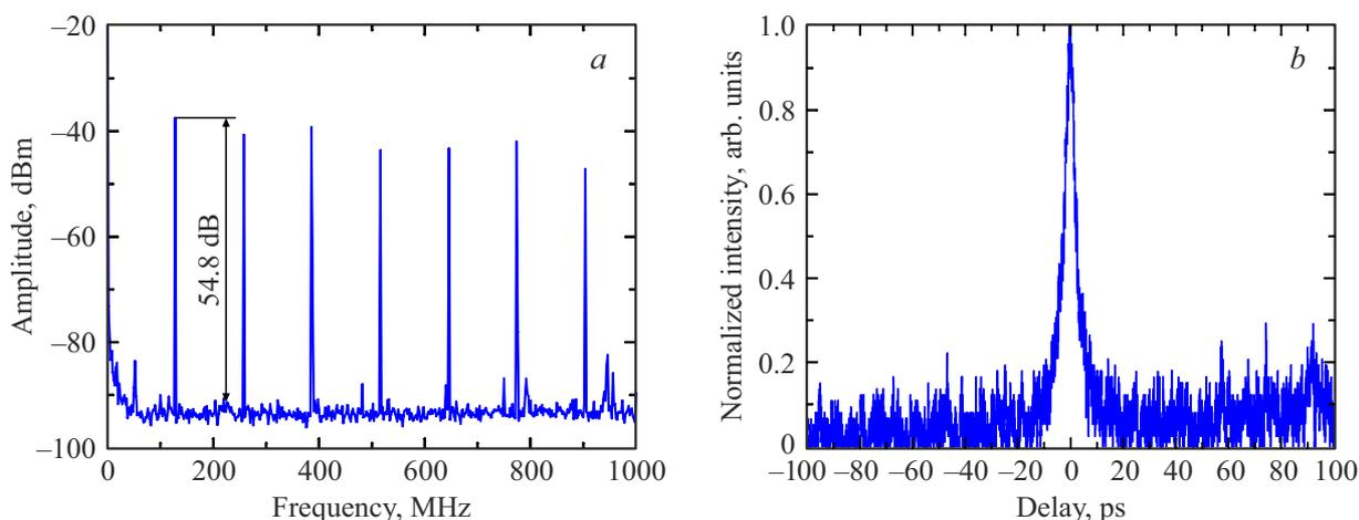
**Figure 2.** RF spectrum (a) and intensity autocorrelation (b) for the single-pulse mode (transmission of the resonator output mirror 2%).
