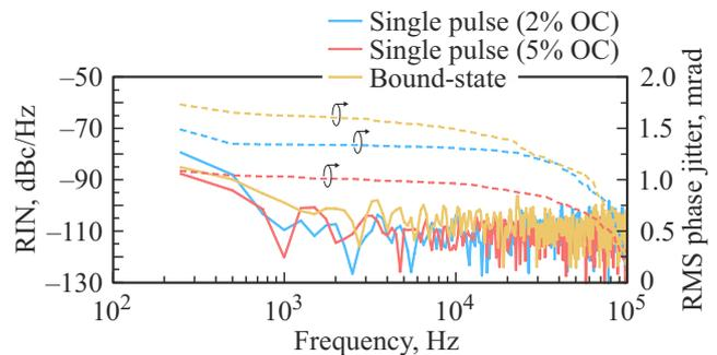
**Figure 6.** Intensity noise measurements for a Cr:ZnSe laser.
