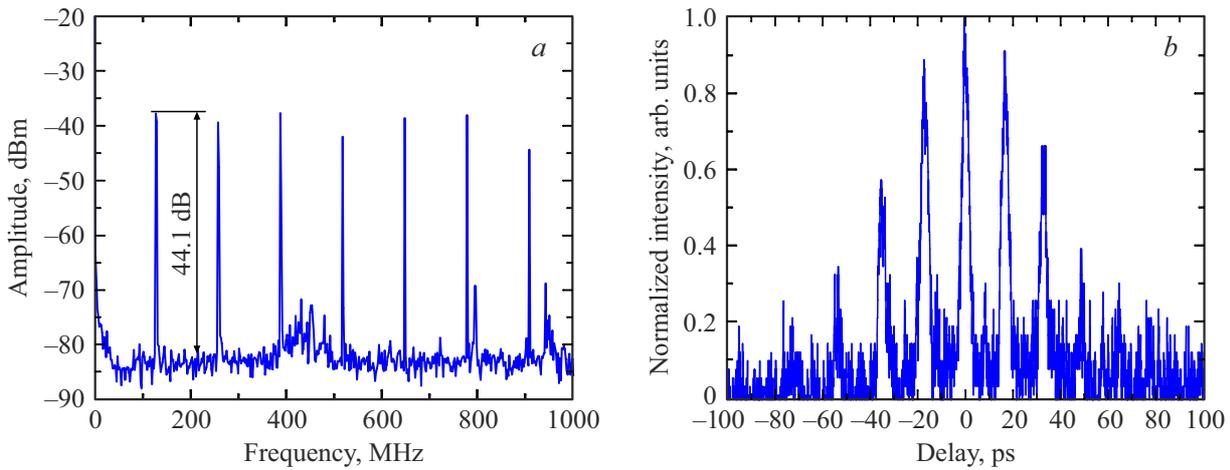
**Figure 4.** RF spectrum (a) and intensity autocorrelation (b) for the bound pulses regime (transmission of the resonator output mirror 2%).
