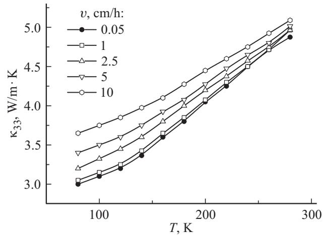
Figure 3. Thermal conductivity vs. temperature of  $\text{Bi}_{0.88}\text{Sb}_{0.12}$  crystals grown at different rates  $v$ .
