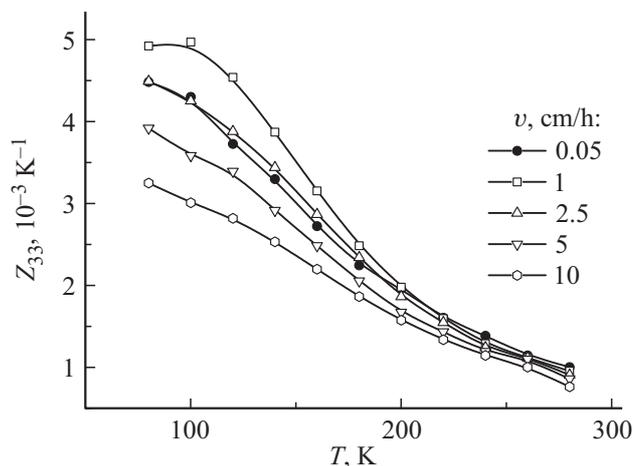
**Figure 5.** Thermoelectric Q-factor vs. temperature of  $\text{Bi}_{0.88}\text{Sb}_{0.12}$  crystals grown at different rates  $v$ .
