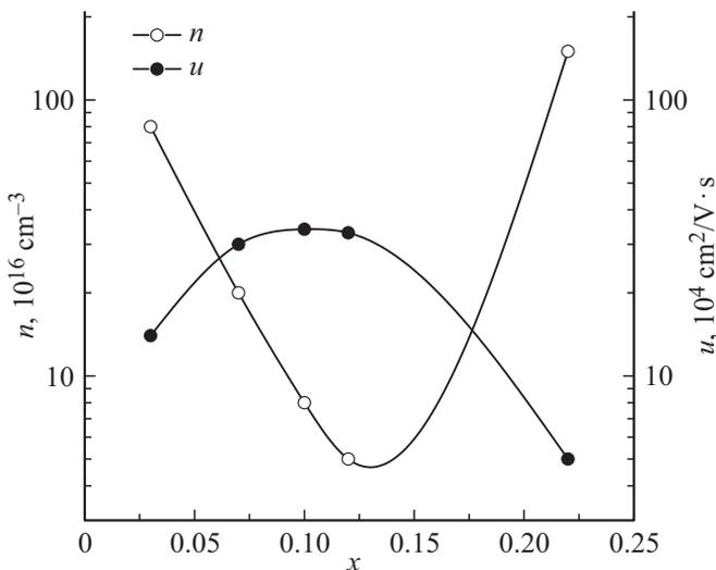
Figure 2. Concentration  $n$  and mobility  $u$  vs. composition of  $L$ -electrons in crystals of  $\text{Bi}_{1-x}\text{Sb}_x$  system.
