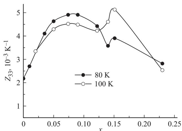
**Figure 6.** Thermoelectric Q-factor  $Z_{33}$  vs. antimony concentration at low temperatures.
