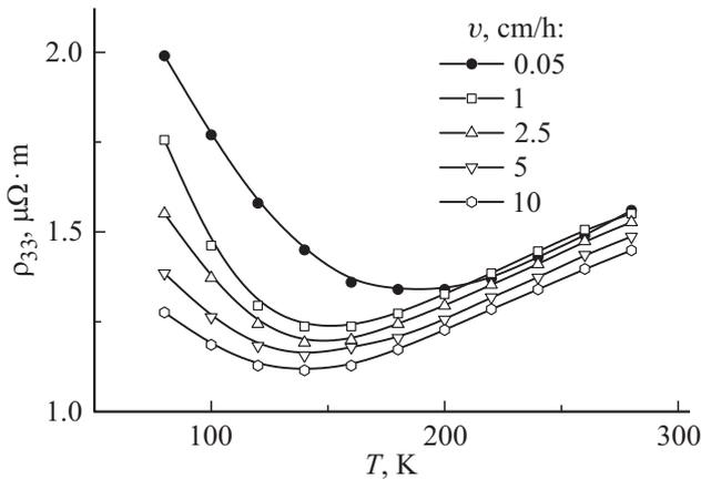
Figure 1. Resistivity vs. temperature of  $\text{Bi}_{0.88}\text{Sb}_{0.12}$  crystals grown at different rates  $v$ .
