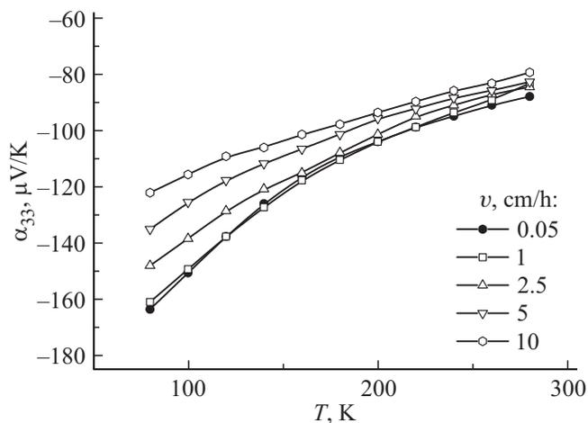
**Figure 4.** Thermoelectric EMF vs. temperature of  $\text{Bi}_{0.88}\text{Sb}_{0.12}$  crystals grown at different rates  $v$ .
