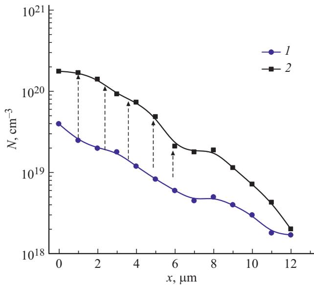
**Figure 3.** Concentration distribution of holes (gallium) in the absence (curve 1) and in the presence (curve 2) of phosphorus.
