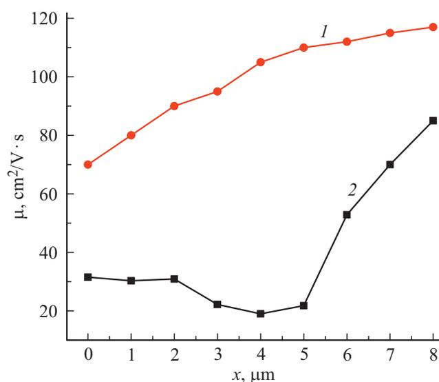
**Figure 5.** Change in electrons mobility in silicon doped with phosphorus (1) and in silicon (pre-doped with phosphorus) doped with gallium (2).
