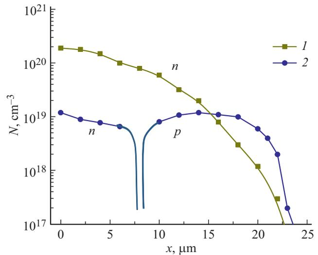
**Figure 2.** Concentration distribution of electrons (phosphorus) in samples additionally annealed at  $T = 1250^\circ\text{C}$ ,  $t = 4$  h (curve 1); concentration distribution of charge carriers in gallium-doped samples pre-doped with phosphorus (curve 2).  $n$ - and  $p$ -type of sample conductivity at a given depth.
