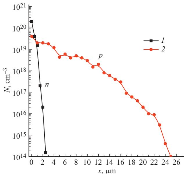
**Figure 1.** Concentration distribution of electrons (phosphorus atoms) and holes (gallium) in the silicon lattice diffused independently of each other: 1 — distribution of electrons (phosphorus) at  $T = 1000^\circ\text{C}$ ,  $t = 2$  h; 2 — distribution of holes (gallium) at  $T = 1250^\circ\text{C}$ ,  $t = 4$  h.
