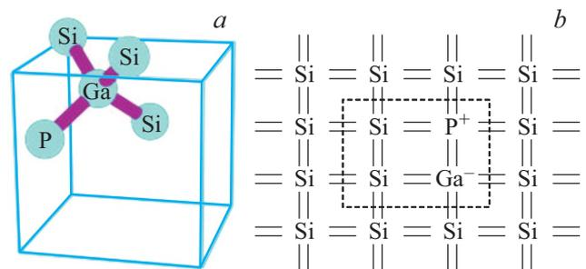
**Figure 4.** Quasimolecules  $\text{Ga}-\text{P}^+$  (a), binary electrically neutral lattices of  $\text{Si}_2\text{P}^+\text{Ga}^-$  type in silicon (b).
