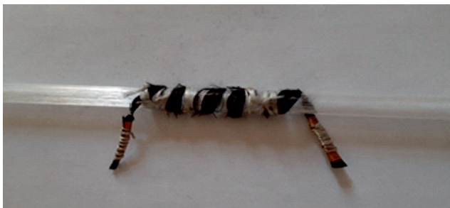
Figure 2. The operating model of thermoelectric generator on p-n junctions of strip CF on a quartz glass tube.
