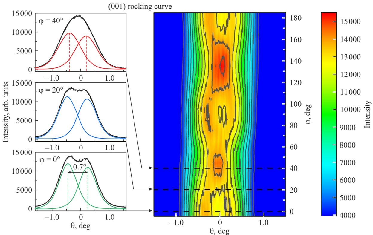
Figure 2. Rocking curves around the (001) reflection of BFO/MgO film recorded at different angles of  $\varphi$ .
