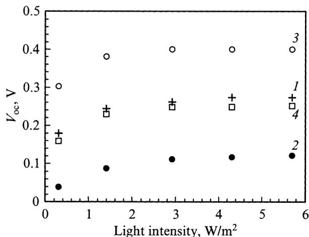
**Figure 3.** Irradiance dependence of open-circuit voltage of the solar cells based on a heterojunction between  $C_{60}$  thin film and different types of Si substrates [34] heavily doped  $p$ -Si (1), lightly doped  $p$ -Si (2), lightly doped  $n$ -Si (3) and heavily doped  $n$ -Si (4).
