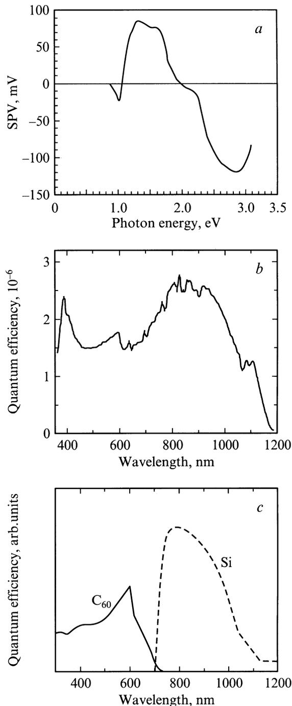
**Figure 2.** Spectral characteristics of the Al/ $C_{60}$ / $p$ -Si/Al solar cells: Surface Photovoltage Spectrum [32] (a); experimental (b) and calculated (c) spectral response.
