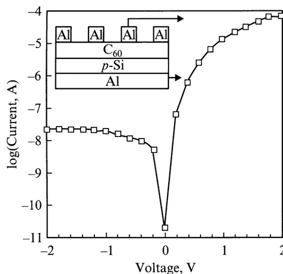
**Figure 1.** Dark  $I$ - $V$  curve of the Al/ $C_{60}/p$ -Si/Al heterojunction solar cell (inset shows a schematic diagram of the device) [32].
