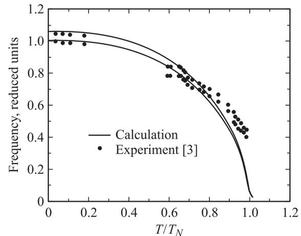
Figure 2. Temperature dependence of AFMR frequencies.
