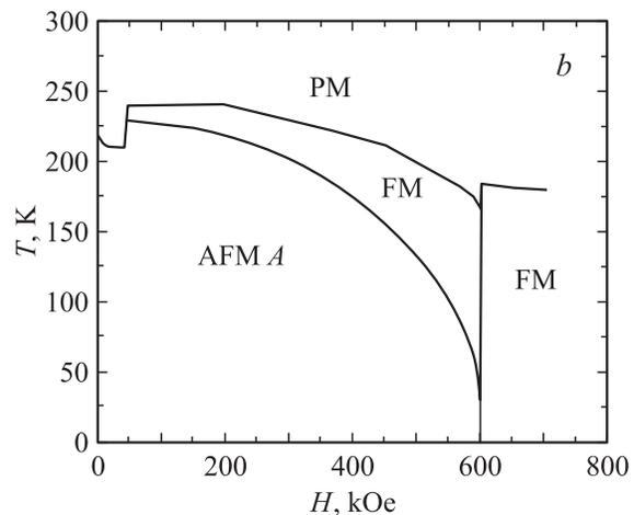
**Figure 4.** Phase diagram  $H$ – $T$ .  $a$  —  $H \parallel x$ ;  $b$  —  $H \parallel y$ . „AFM  $A$ “ is the  $A$ -type antiferromagnet.
