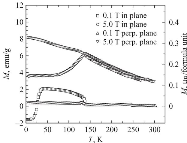
**Figure 3.** Temperature dependence of total magnetization. Experimental data are taken from paper [6].
