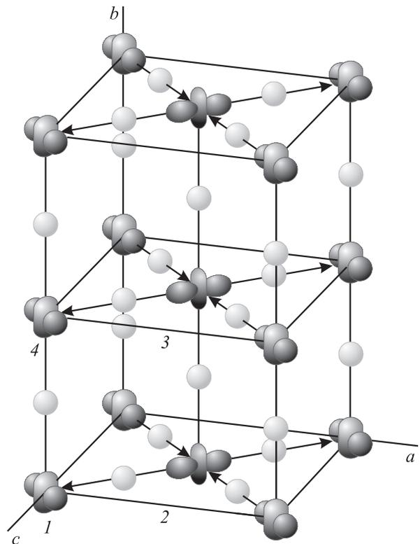
**Figure 1.** Crystal and orbital structures. Lanthanum ions are omitted. Manganese ions are drawn as  $e$ -orbitals. Arrows show  $e$ -type distortions of oxygen octahedral. Numbers enumerate orbital and magnetic sublattices.
