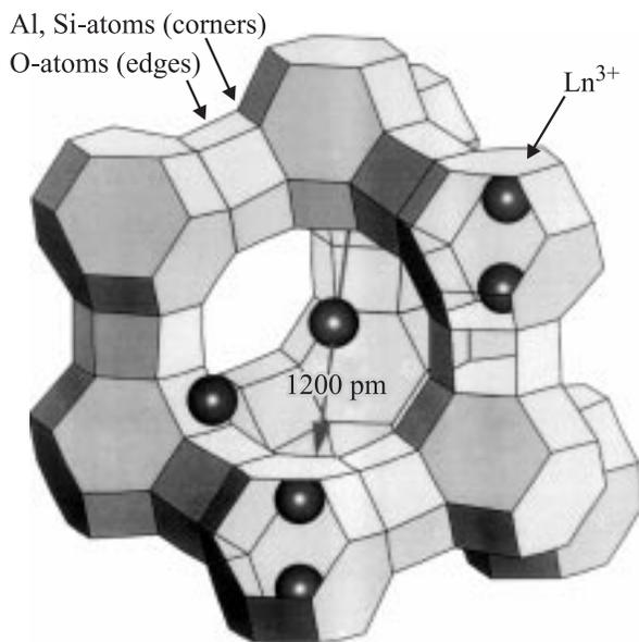
**Figure 1.** Sketch of the Faujasite structure (zeolite X). Cation sites are indicated by spheres. Positions outside of the cuboctahedral sodalite cages are not occupied in the zeolites X discussed in this report.
