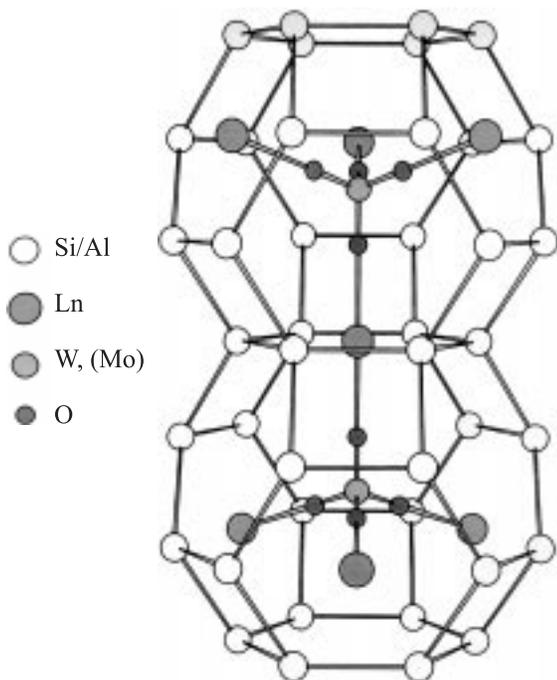
**Figure 4.** Structure of sodalite with included rare earth tungstates  $[\text{Ln}_4(\text{Al}_8\text{Si}_4\text{O}_{24})(\text{WO}_4)_2]$ .
