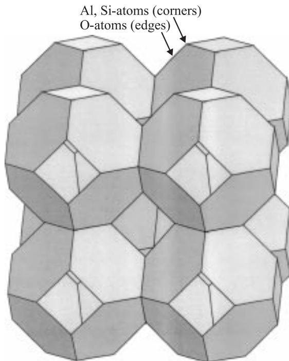
**Figure 2.** Simplified sketch of the sodalite structure.
