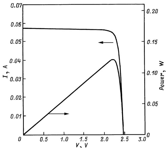
**Figure 6.** Light current–voltage and power–voltage curves of the high-efficiency InGaP/GaAs tandem cell measured at the Japan Quality Assurance Organization: cell area  $4\text{ cm}^2$ , AM 1.5,  $100\text{ mW/cm}^2$ ,  $25.3^\circ\text{C}$ , short-circuit current  $I_{sc} = 56.88\text{ mA}$ , open-circuit voltage  $V_{oc} = 2.488\text{ V}$ , fill-factor  $FF = 85.6\%$ , efficiency  $30.3\%$ .
