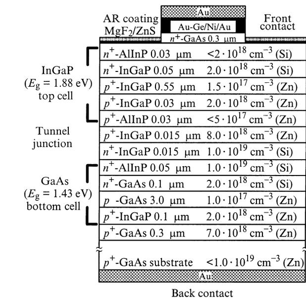
**Figure 5.** A schematic cross-section of the high-efficiency InGaP/GaAs 2-junction cell.
