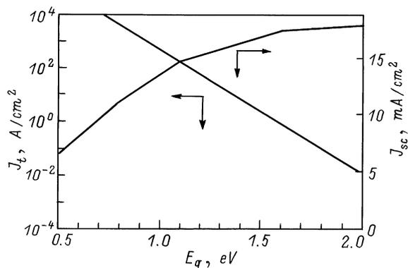
**Figure 2.** Calculated tunnel peak current density ( $J_t$ ) and short-circuit current density of GaAs bottom cell ( $J_{sc}$ ) as a function of bandgap energy ( $E_g$ ) of the tunnel junction.
