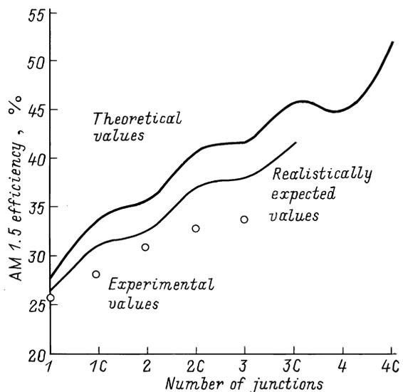
**Figure 7.** Theoretical and realistically expected conversion efficiencies of single-junction and multi-junction solar cells in comparison with experimentally realized efficiencies.  $C$  indicates concentration.
