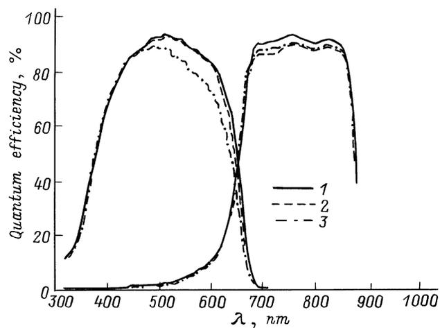
**Figure 3.** Spectral response of the InGaP/GaAs tandem cells dependent on their tunnel junction structures: 1 — AlInP/InGaP, 2 — AlInP/GaAs, 3 — InGaP/GaAs. All the tunnel junctions have DH structure.
