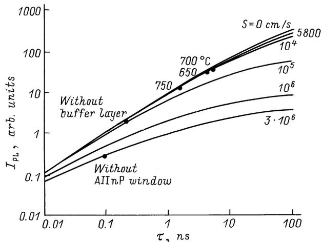
**Figure 1.** Changes in photoluminescence intensity ( $I_{PL}$ ) of the solar cell active layer as a function of the minority carrier lifetime ( $\tau$ ) of the  $p$ -InGaP base layer and surface recombination rate ( $S$ ). Values of the growth temperature and the surface recombination rate are shown.
