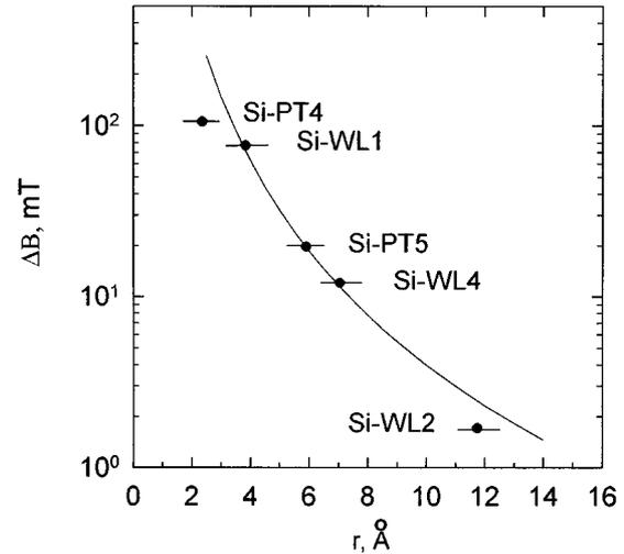
**Figure 3.** Dependence of the fine structure splitting  $\Delta B$  on the distance  $r$  between two interacting electrons.
