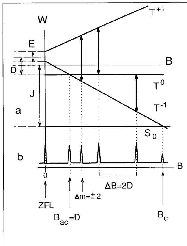
Figure 1. Energy levels of a system of two electrons in a magnetic field  $B$  (a) and the expected positions of the SDR detected EPR spectra of the change of the microwave photoconductivity (b).
