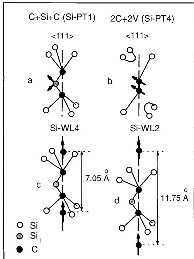
**Figure 4.** The models of the carbon related defects corresponding to the SDR-EPR spectra Si-PT1 (*a*), Si-PT4 (*b*), Si-WL1 (*c*), and Si-WL2 (*d*).
