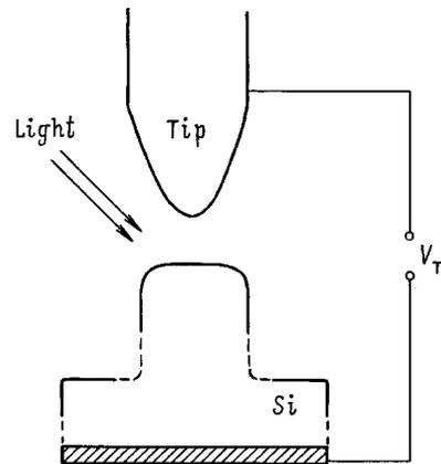
**Figure 1.** Schematic representation of a tungsten tip of a scanning tunneling microscope placed above an illuminated nanoparticle (column) of porous Si. The top of a nanoparticle, covered with an oxide layer, is separated from the bulk Si by a poorly conducting region of porous Si. Below the nanoparticle the bulk of the specimen with aluminized back side (shaded) is schematically depicted.  $V_T$  is the external voltage applied between the tip and the aluminized back side.
