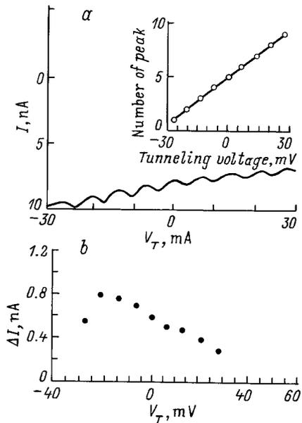
**Figure 2.** *a)* Oscillation of the tunneling current  $I$  between the STM tip and porous Si surface illuminated at  $\lambda = 647$  nm from the Kr/Ar laser, when the value of  $V_T$  is changed. *b)* Dependence of the amplitude  $\Delta I$  of the current modulation on the voltage  $V_T$ .
